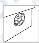
2. unscrew the lid by rotating it anticlockwise (see figure): a little water may trickle out. This is perfectly normal;
