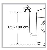
Connect the drain hose, without bending it, to a drain duct or a wall drain situated between 65 and 100 cm from the floor;
