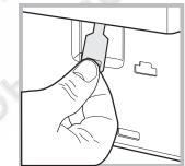
4. pull outwards using the tab as indicated in the figure, until the plastic tie-rod is freed from its stop position; pull downwards and open the door at the same time.5. reposition the panel, making sure the hooks are securely in place before you push it onto the appliance.
