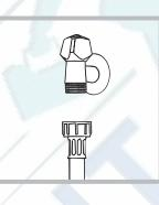
1. Connect the inlet hose by screwing it to a cold water tap using a 3/4 gas threaded connection (see *figure*). Before performing the connection, allow
